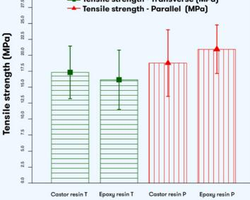
The results indicate a close resemblance in tensile strength values between composites with tururi fibers arranged transversely: 17.33  $\pm$  4.12 MPa (Material 1) and 16.18  $\pm$  4.65 MPa (Material 2). Comparable values were observed for composites with tururi fibers arranged in parallel: 18.78  $\pm$  5.22 MPa (Material 1)and 20.95  $\pm$  3.80 MPa (Material 2).
