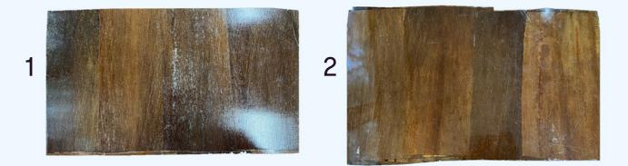
For density measurement, the results were  $0.79 \pm 0.04$  g/cm<sup>3</sup> (Material 1) and  $0.91 \pm 0.20$  g/cm<sup>3</sup> (Material 2). Lower density values are advantageous for polymer composites as they indicate the potential for lighter materials. The moisture content results were 5.30 ± 0.30% (Material 1) and 4.90 ± 0.60% (Material 2).
